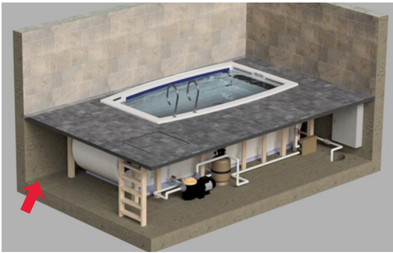
Concrete slab with retaining walls. See #3 above
