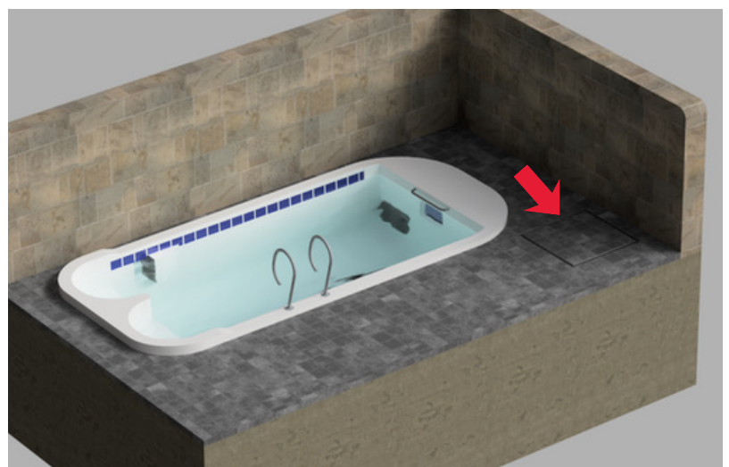
Hatch opening in finished decking to access pit. See #7 above
